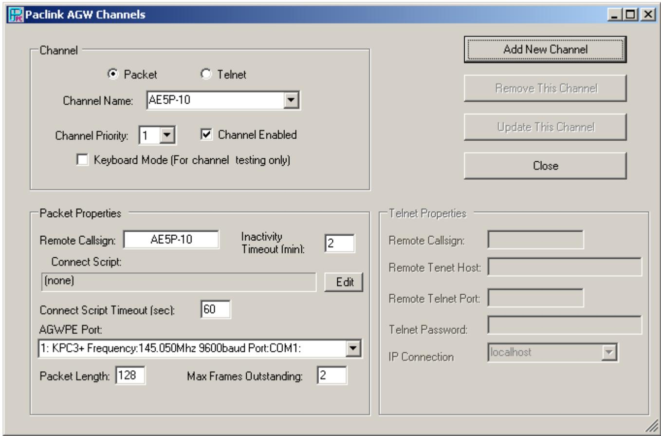
Click on Packet, then enter a Channel Name: (for Nacogdoches, we are using AE5P-10, for Lufkin, use W5IRP-10)
